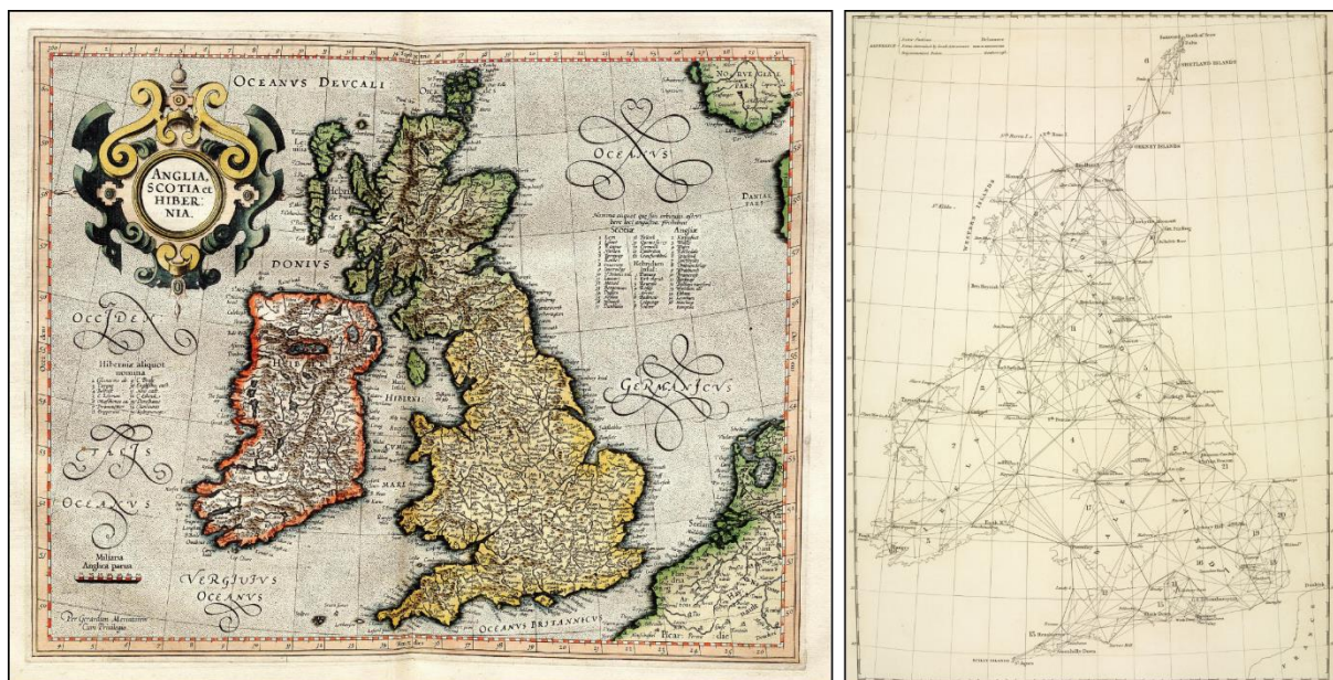
Figure 1: Maps of Great Britain and Ireland before triangulation ( left: Atlas Cosmographicae by Gerardus Mercator, 1512 – 1594) and after triangulation ( right: Principal Triangulation of Britain, 1791 – 1853). While triangulation was used for local mapmaking prior to this date, with the earliest evidence for the technique dating to ~1000 AD, this was the first attempt to apply the technique to an entire country.
